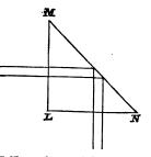
they come out through the face LN nearly at right angles to it, and proceed to form the image p'q' as in Art. 383. It appears from experiment that the loss of light, by the two refractions and the total reflection in the prism, is less than the loss by the single reflection at the surface HK of Art. 383.
