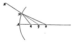
may be given in the same words as in that Article; but in applying the Rule we must remember, what the diagram shews, that AQ and AQ are now less than AO. For example, suppose as before that AO is 12 inches, and the index of refraction  $\frac{4}{3}$ ; and let AQ be 6 inches. Then
