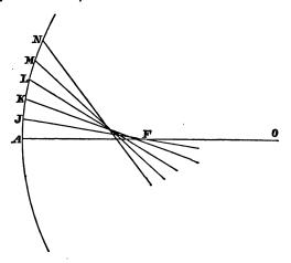
reflected ray with the axis. The intersections with each other of successive reflected rays in the plane of the paper give an assemblage of points which may be considered to form a curve; this curve is called a caustic. The reflected rays in the diagram are all drawn from the part of the reflector which is above the axis, and the corresponding part of the caustic is above the axis. If we suppose the
