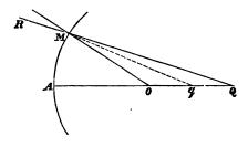
centre of the sphere, OA the axis of the refractor, A the vertex. We will suppose the origin of light to be further from the vertex than O is; let it be at Q in AO produced. Let QM represent one of the rays, incident at M on the spherical refracting surface; and let MR be the direction of the ray after refraction. Produce RM to meet the axis at q. Join OM. Then QMO is the angle of incidence,
