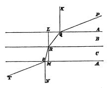
again; and let these media be separated by parallel plane surfaces. Draw QK, LRM, and SN respectively at right angles to the plane surfaces. Then these three straight lines are all parallel; and therefore the angle LRQ is equal to the angle between RQ and KQ produced, and the angle SRM is equal to the angle between RS and RS
