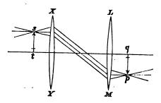
which is *inverted* with respect to pq, and therefore erect, with respect to the original object; and this image may be viewed through an eye glass, and so magnified, in the usual way.
