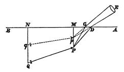
PQ be an object placed before a plane refracting surface AB; we will suppose that on the other side of AB there is a vacuum, or a medium having a less refractive index than
