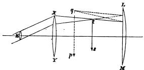
field lens and the eye lens: this image is therefore at a distance from XY equal to the focal length of XY. Thus rays which diverge from t and fall on XY, will after refraction by XY form a pencil parallel to the straight line joining t with the centre of XY. Thus to an eye at E which is adapted for the reception of parallel rays such rays will form an image of the point t; and in this way the eye will perceive an image of the whole object.
