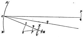
wards the reflector. Then by the aid of an eye glass he examined the image formed by the concave reflector, so that he did not have to shift the position of this image, as in the other reflecting telescopes, and thus he avoided the loss of light caused by this shifting. In order to prevent the head and shoulders of the observer from intercepting too much of the light falling on the concave re-
