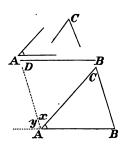
63. To construct a triangle, having given a side, an angle at the side, and the opposite angle.
