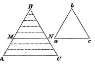
a small line which is contained in each of them a certain number of times exactly, let this be marked off along them, and be contained, for example, p times in BA and q times in BM; we then have
