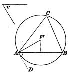
the chord and the tangent at A, as it is measured by the same arc; therefore make  $\angle BAD = \angle v$ , and the centre may then easily be found. For as AD must be a tangent, the centre must lie in the perpendicular AF on AD, and therefore lie where this cuts a perpendicular on the middle point of the chord. If the given angle is a right angle, the arc will be a semicircle.
