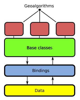
Data bindings are the mechanism used by SEXTANTE to conect the algorithms to differents data sources. Using this, SEXTANTE can run on many different GIS and can provide
